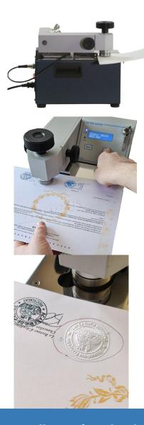
This electric embossing machine is an advanced device designed for the rapid and efficient embossing of official documents and other materials. Equipped with a powerful electric motor, the T2E offers reliable and consistent performance, significantly reducing the manual effort required to perform the operation. Its sturdy and well-built structure ensures stability during use, while the ergonomic design ensures comfortable handling.
