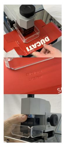
The T2E/M is a dry marking electric machine designed to encode production and expiry dates, batches, and more on packaging in various sectors.
