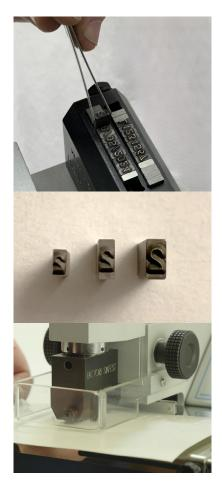
The marking process can be initiated in three ways: the operator can touch the microswitch with the inserted case (which automatically starts the operation), or press the start button, or use an optional pedal.
